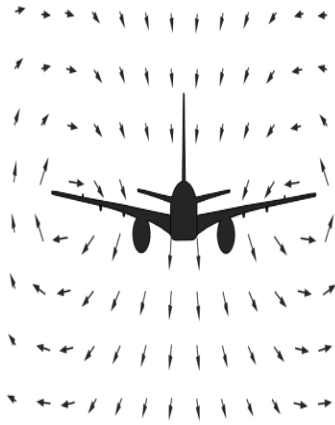
Figure 3.1. Velocities in a crossflow plane behind a lifting wing
