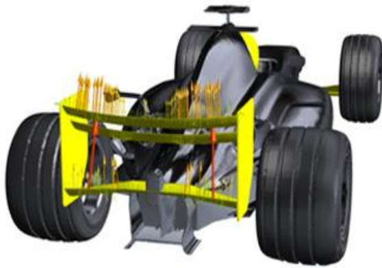
FIG :ANSYS Fluent adjoint solver indicates the necessary shape changes to ensure maximum down force for a race car
