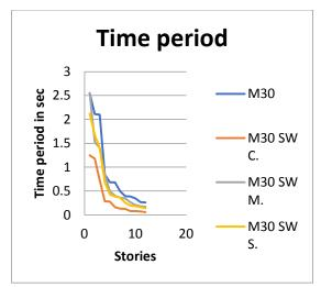
FIGURE 4.6: time period of buildings with shear wall at different positions for M 30 grade of concrete
