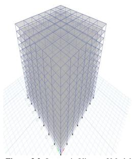
Figure 3.2: Isometric Views of Models Model 2 In zone IV explores a 14-story RC framed skyscraper. The structure has a 42 x 42 m layout with a 3 m average story height. There are seven X-bays and seven Y-bays in all. The constructions had a total length of 40.8 meters.
