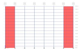
Figure 3.5: Elevation view of the model The third model uses a 14-story RC framed skyscraper in Zone IV for research. On the plan, the building has an area of 42 42 m2 and a typical floor height of three meters. There are 7 berths in the X direction and 7 bays in the Y direction. There was a total of 40.8 meters of height in the constructions.
