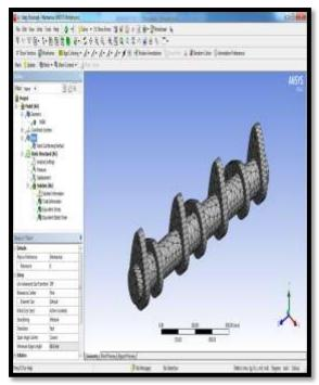
Select static structural right click on  $\rightarrow$ insert  $\rightarrow$  pick rotational velocity and stuck assist  $\rightarrow$  Select displacement  $\rightarrow$  select required area  $\rightarrow$  click on practice  $\rightarrow$ positioned X,Y,Z factor  $0 \rightarrow$
