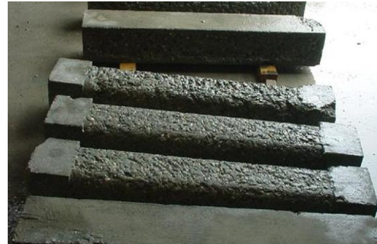
Figure: Surface preparation using pneumatic concrete chisel
