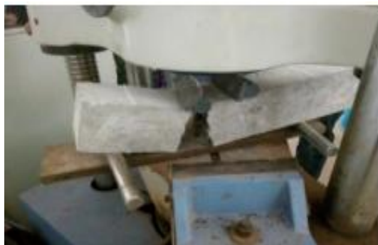
Figure: Flexural strength test
