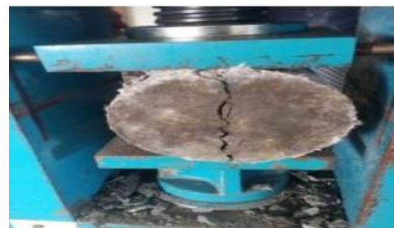
Figure: Split tensile test
