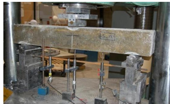
Figure: Beam test setup under quasi-static loading
