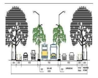
Detailed BRTS section showing segregated footpath, cycle track and motor vehicle lane
