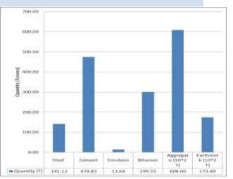
Construction of 1 km NH involves significant consumption of aggregates (coarse/fine); about 60 thousand tonnes of aggregates are consumed per km. Construction substantial also involves
