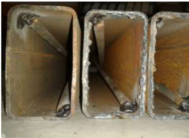
Figure: Shear connector welded specimens
