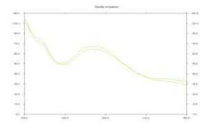
**Fig:9b** In situ HPTLC spectral overlain of Gallic acid obtained from standard and commercial Formulation
