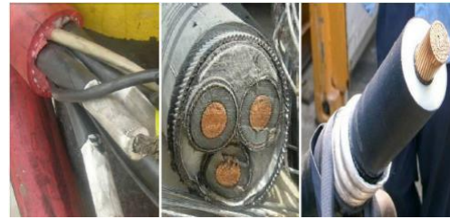
Figure.-core EPR, incl. 3-core XLPE 11kV 1-core XLPE 115kV Data line, radial type
