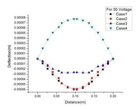
**Fig 12:** Centerline deflection for P=100N/m<sup>2</sup>, V=50 for number of cases
