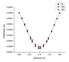
Fig 7: Centerline deflection of plate  $[p-45/45]_{as}$ P=100N/m<sup>2</sup>, V=0,30,50
