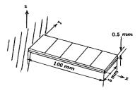
Fig 4: Piezoelectric PVDF BIMORPH BEAM.
