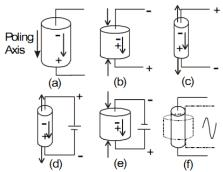
Fig 1.1: Piezoelectric effect
