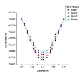
**Fig 10:** Centerline deflection for P=100N/m<sup>2</sup>, V=0 for different cases
