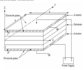
Fig2: Piezoelectric effect
