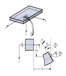
**Fig3**: Un-deformed and distorted geometries of rim of plate based on the assumptions of the first-order plate theory.
