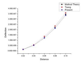
**Fig 5:** PVDF Bimorph Beam's Deflection (for a unit voltage) (m)
