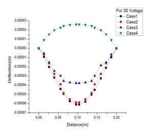
**Fig 11:** Centerline deflection for P=100N/m<sup>2</sup>, V=30 for different cases
