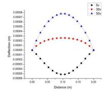
Fig 10: Centerline deflection of plate [p-45/45]<sub>as</sub>P=100N/m<sup>2</sup>, V=0.30.50
