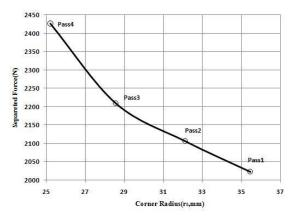
Figure 6. Separated force versus tube corner radius.
