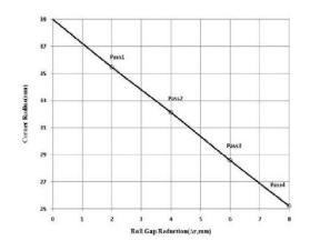
Figure 8. Corner radius versus roll gap reduction.
