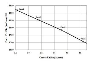
Figure 5. Power dissipated versus tube corner radius.
