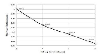
Figure 7. Final rolled tube thickness versus roll gap reduction.
