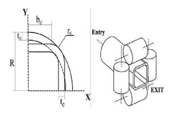
Figure 1. Shape rolling process deformation zone.
