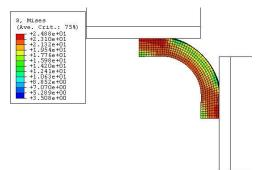
Figure 2. Tube deformed shape after passing through rolls.
