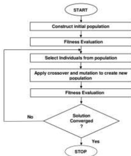
Figure: 4-Flowchart for calculating capacitor size using genetic algorithm
