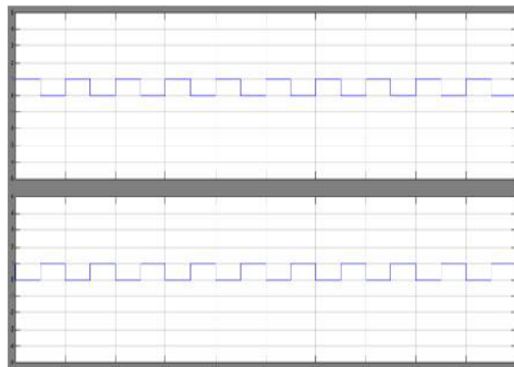
Fig. Gate signal of S5 and S6
