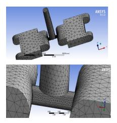
Fig.2.1: Meshed model Fig. 2.2 Zoomed Meshed Model at the Gates
