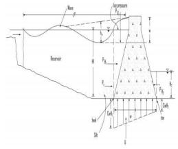
Figure 3.2 - Forces Acting on a Gravity Dam
