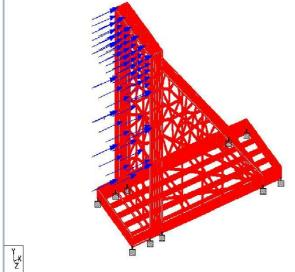
Figure 5.18 wind direction x with 15KN-.m
