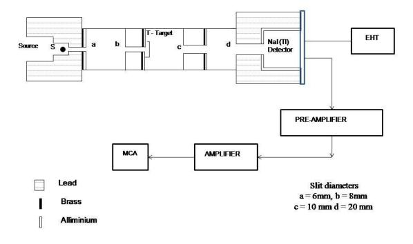
Figure 1. Schematic Diagram of Narrow Beam Geometric Setup.
