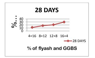
Split tensile strength N/mm<sup>2</sup> Vs percentage of FLYASH and GGBS at 7 days and 28 days
