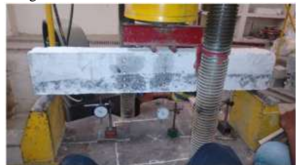
Fig: Test set up of a beam testing under flexure
