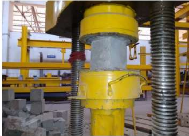
Fig: Cubes testing in universal testing machine for compressive strength
