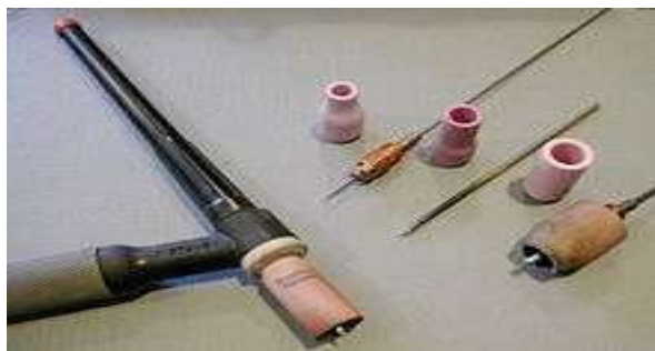
Figure GTAW torch with various electrodes, cups, collets and gas diffusers
