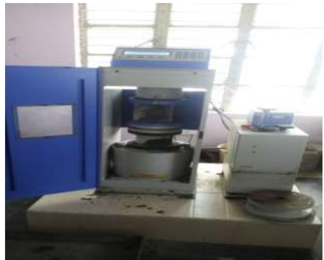
Figure: Compressive testing machine.
