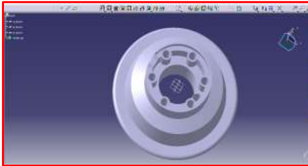
Figure: The Wheel hub developed in Catia.
