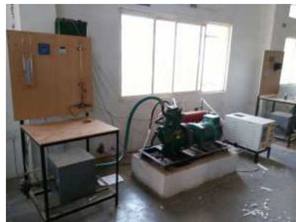
Figure: 4-stroke diesel engine with electrical loading
