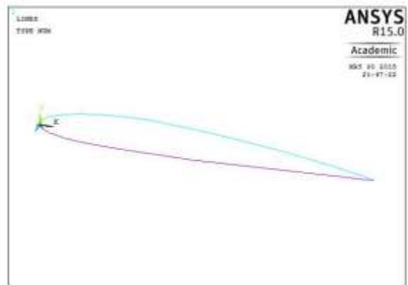
Figure: Profile of NACA 2412 airfoil model
