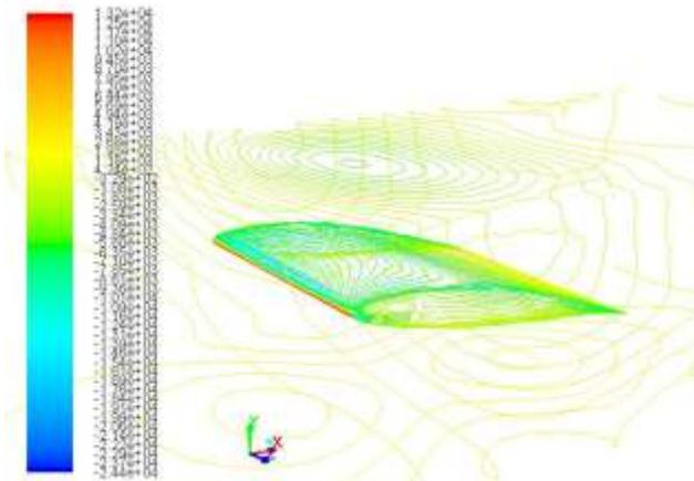
Figure: Pressure contours on the airfoil model
