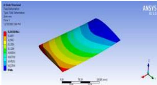
Fig: Total deformation of the airfoil model
