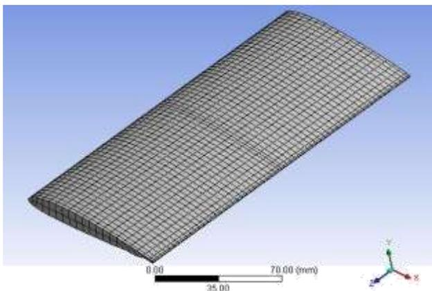
Figure: 3D Meshed model of airfoil
