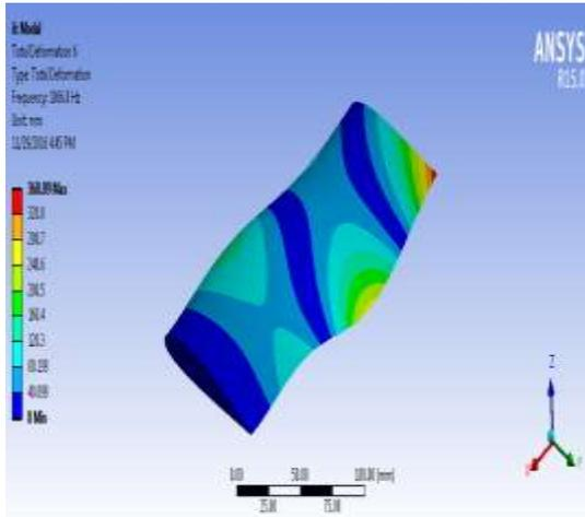
Fig: Sixth mode shape of the airfoil model
