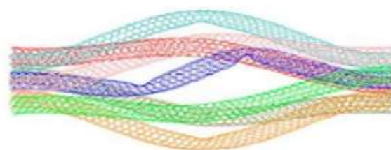
Bending deformations of SWCNT bundle under axial compression
