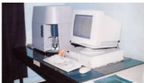
Malvern particle size analyzer (Model Micro-P, range 0.05-550 micron).
