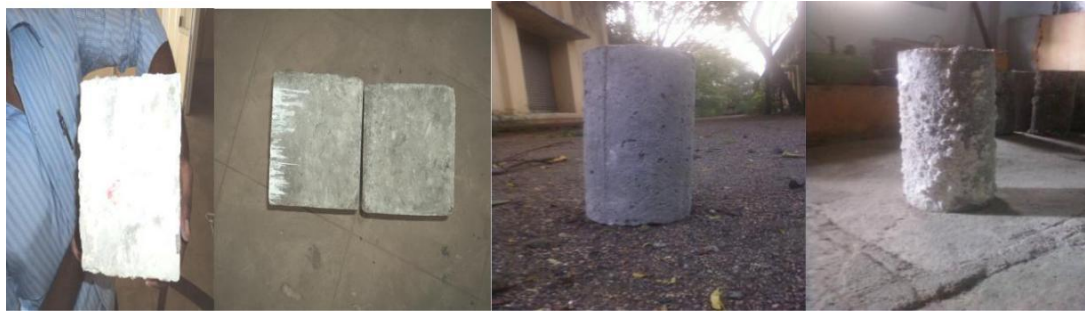
Figure 5: GPC and PPCC specimens exposed to magnesium sulphate solution after 45 days
