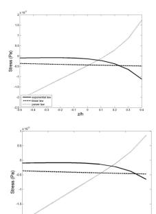
Stress distribution along the thickness for exponential material and temperature
