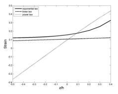
Stress distribution and Strain variation according to the temperature for exponential material and temperature distribution, linear material distribution and linear temperature and power law material distribution.
