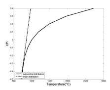
Comparison of temperature distribution along the thickness according to FDM and power law
