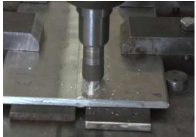
Fig 4: Friction stir welding process
