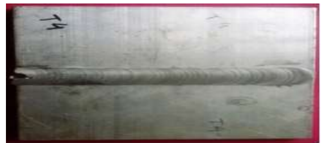
Fig 8: Doublepass with triangle
