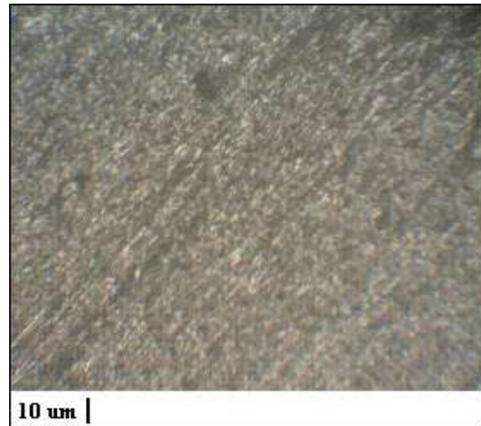
Fig 20: Single pass with triangle tool
