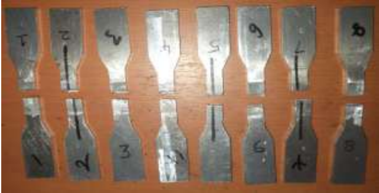
Fig 16: Fractured specimens after tensile test
