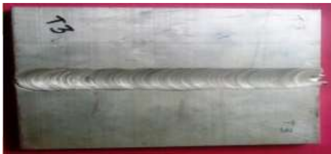
Fig 7: Doublepass with conical tool
