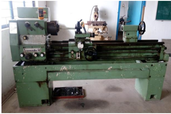
Fig 2.3: TURN MASTER-40 Engine Lathe
