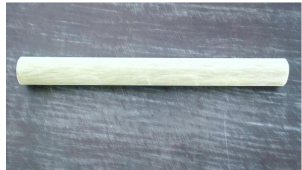
Fig 2.1: GFRP Composite bar Specimens
