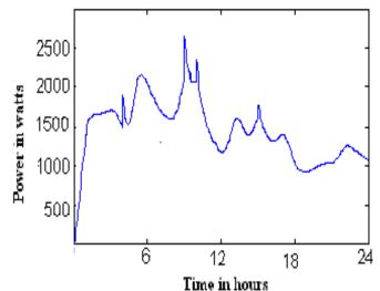
**Figure 13.Power output using Hybrid Method (Variable Load)** When Hybrid method is employed for the MPPT for variable load Maximum power is 2548 W, Average power is 1.025kW and energy attained from the WECS on complete day is 24.62kWh.
