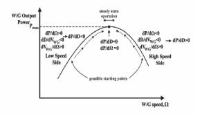
Figure 4.MPP tracking process.
