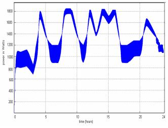
Figure 8. Power output without MPPT.
