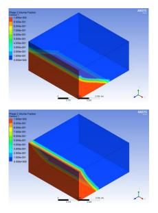
Fig.4.5 Volume fraction of liquid at 1.3sec Fig.4. 6Volume fraction of liquid at 1.8sec
