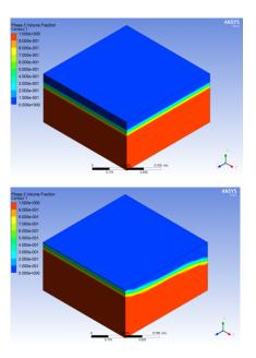
Fig.4.9 Volume portion of liquid at 0.01sec Fig.4.10 Volume portion of fluid at 0.1sec.
