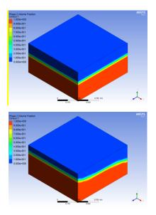
Fig.4.1 Volume portion of fluid at 0.005sec, Fig.4.2 Volume portion of liquid at 0.1sec.
