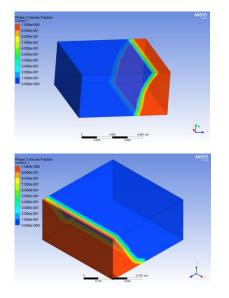
Fig.4.3 Volume portion of fluid at 0.7sec Fig.4.4 Volume portion of fluid at 1sec
