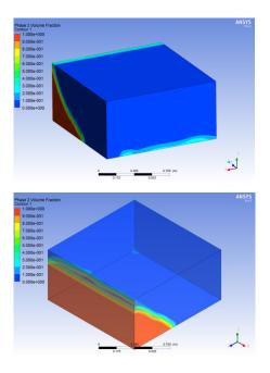
Fig.4.13 Volume portion of fluid at 1.8sec Fig.4.14 Volume portion of liquid at 2.5sec
