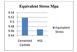
Comparison of Total Deformation and Equivalent Stress for cemented carbide and HSS
