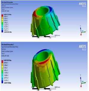
**Deformation along X Axis for cemented carbide material tool:** The figure shows the variation of Directional Deformation along Y axis in mm, The maximum deformation of magnitude 0.00012mm was observed. **Deformation along Y Axis for cemented carbide material tool :** The figure below shows the variation of Directional Deformation along Y axis in mm, The maximum deformation of magnitude 1.37 e-05 mm was observed.
