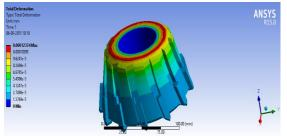
The figure below shows the variation of Directional Deformation along X axis in mm, The maximum deformation of magnitude 0.000121mm was observed.
