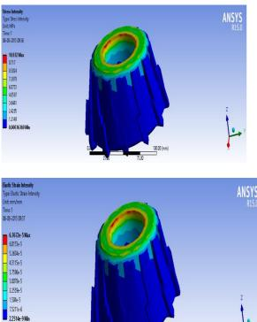
**Stress Intensity for HSS Tool :** Figure shows the variation of strain intensity for the tool
