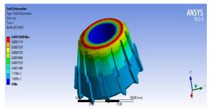
The figure shows the total deformation of the tool under the moment applied for High Speed Steel material, Maximum deformation was observed at the top face of the tool with magnitude of 0.00035.
