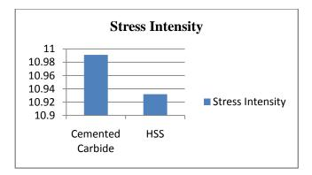
Comparison of Stress intensity for cemented carbide and HSS
