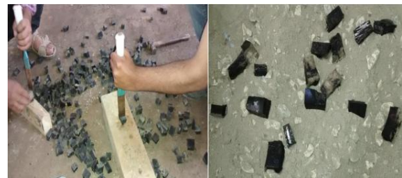
Figure 1.1: Manual cutting of tyre rubber to the size of coarse aggregates Scrap tyres:
