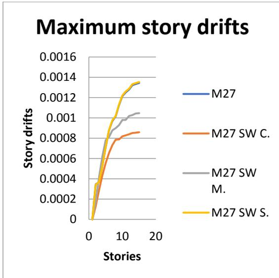
**Figure 4.8:** Drift of buildings with shear wall at different positions for M 27 grade of concrete
