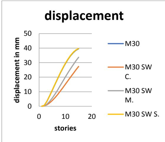
**Figure 4.4:** Displacements of buildings with shear wall at different positions for M30 grade of concrete
