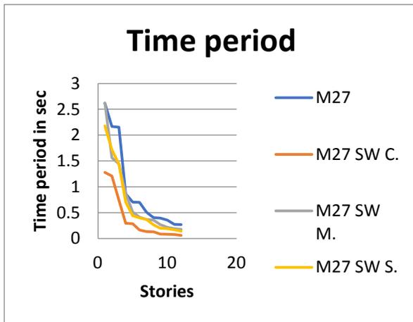
**Figure 4.9:** time period of buildings with shear wall at different positions for M 27 grade of concrete
