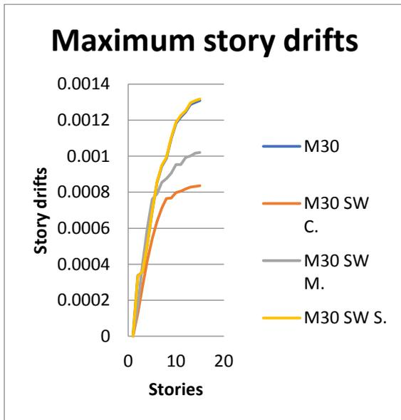
**Figure 4.5** Drift of buildings with shear wall at different positions for M30 grade of concrete
