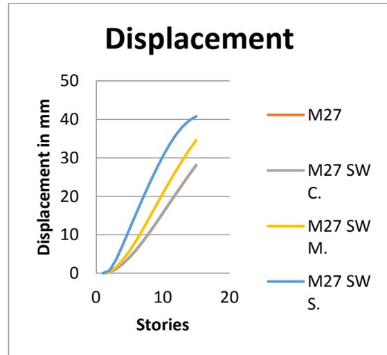
**Figure 4.7:** Displacements of buildings with shear wall at different positions for M27 grade of concrete
