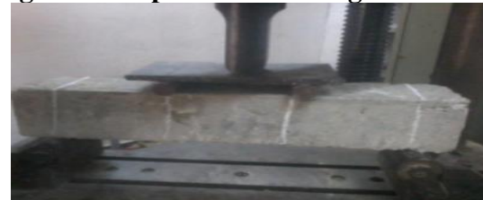
Figure 3.6: Specimen under Flexural Strength Test
