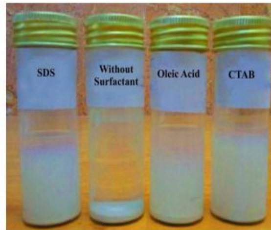
Fig. 4 Effect of surfactant on Mg(OH) 2 / water nanofluid (after 45days)
