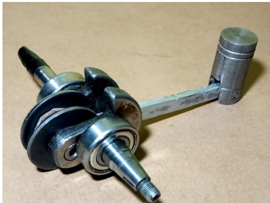
Figure 5: Comprising Piston & Pin, Connecting Rod, Crank Shaft, Bearing, Washer & Pin
