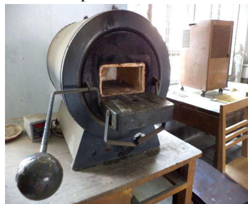
Fig.1.2 Heat Treatment Furnace
