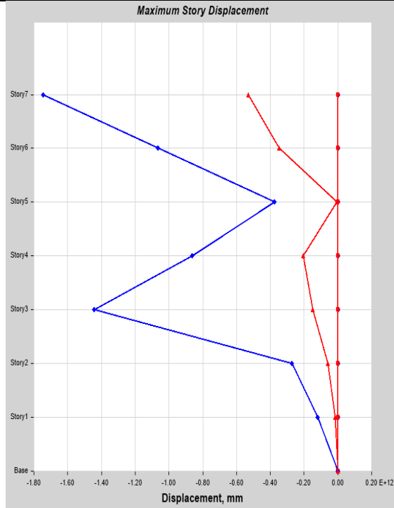
Figure: Story displacement of conventional concrete in zone III in X-direction & Y- direction
