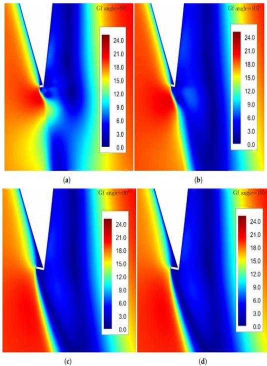
**Figure: Total velocity plot (in m/s) in the rotating frame of reference at a tip speed ratio of  $\lambda = 2.13$ . (Top): GF height of  $0.5\%c$  in (a,b), (middle): GF height of  $1\%c$  in (c,d),**
