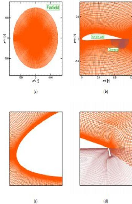
Figure: Computational mesh of the static airfoil and applied boundary conditions. (a) Overall mesh, (b) enlarged views near the airfoil (c) near the leading edge and (d) near the trailing edge.
