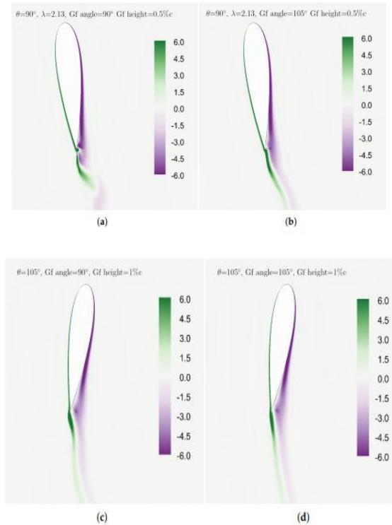
**Figure: Spanwise vorticity contour at a tip speed ratio of  $\lambda = 2.13$ . (Top): GF height of  $0.5\%c$  in (a,b), (middle): GF height of  $1\%c$  in (c,d).**
