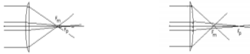
FIG 4: Plano-convex lens by arranging convex side facing the incident or emergent rays
