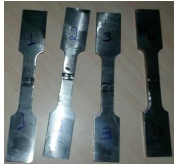
Fig 3.3 standard specimen for tensile test
