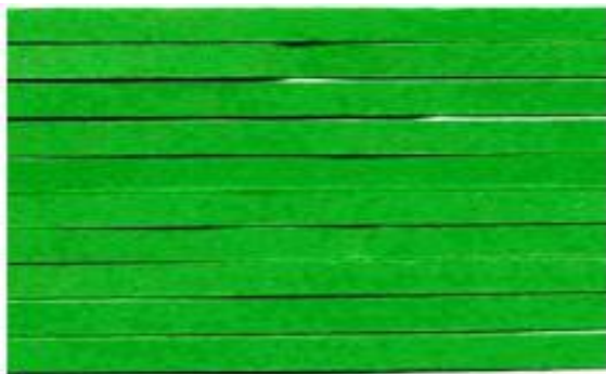
Fig.1: Structure of the Unidirectional (UD) Continuous CFRP Composite Material.
