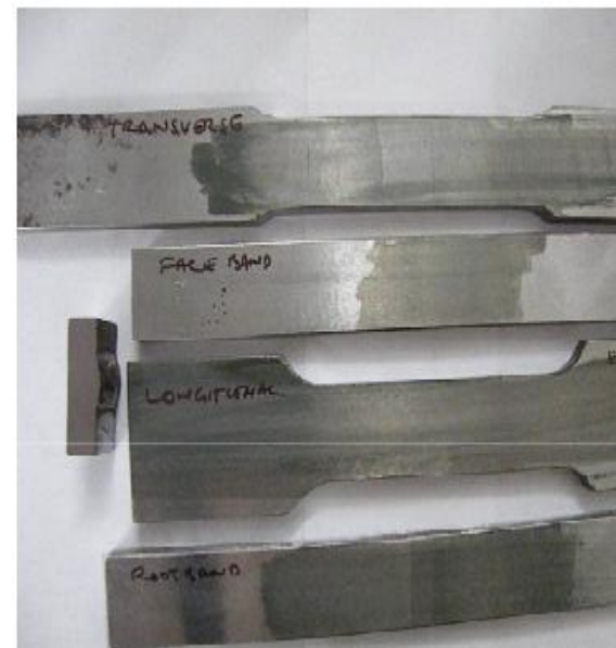
Testing Samples of Base Material before Tensile, Yield Testing and Face and Bend Root Tests
