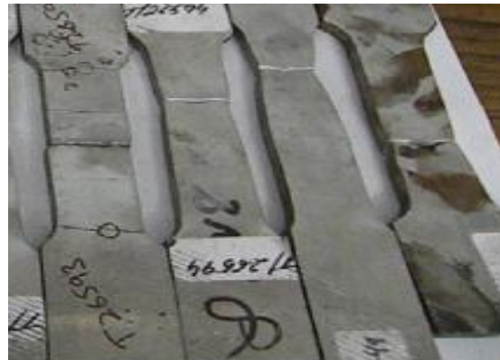
Broken Test Samples after Yield, Tensile and Bend Tests
