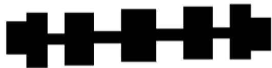
Figure(5) The design of ninth order low pass filter is as shown
