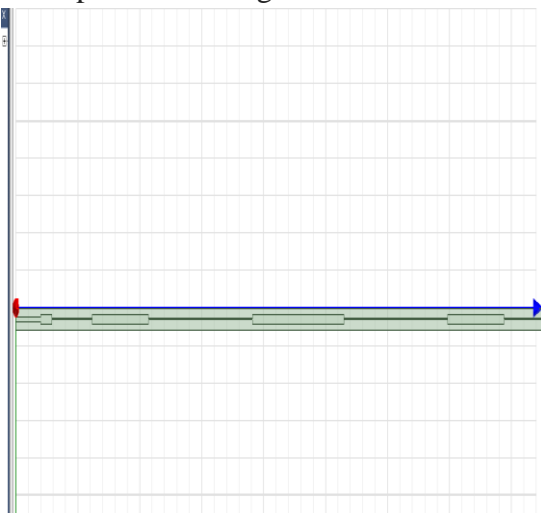
Figure (7) Top View of HFSS layout design of order low pass filter
