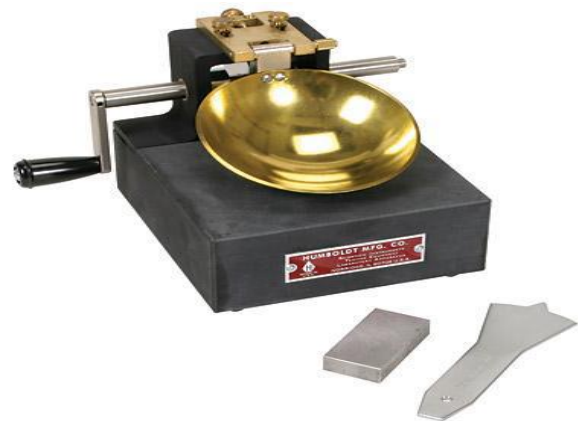
FIG.2: Liquid Limit Apparatus Observations & calculations (sample 1):
