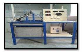
Fig 4.1 Experimental setup of a heat pipe.
