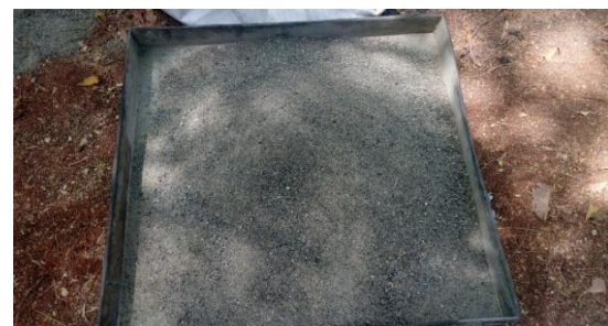
FIG 1. AIR-COOLED BLAST FURNACE SLAG IN FINE AGGREGATE FORM
