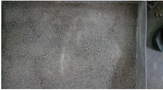
FIG 2. GRANULATED BLAST FURNACE SLAG
