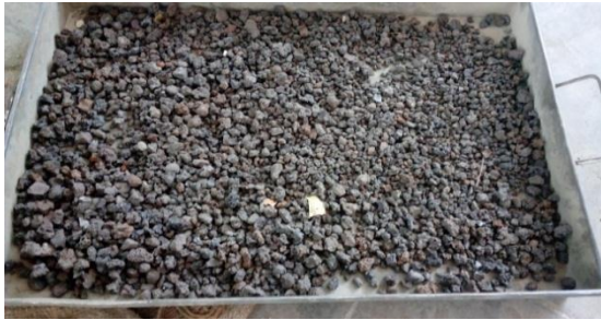
FIG 3. STEEL SLAG IN COARSE AGGREGATE FORM
