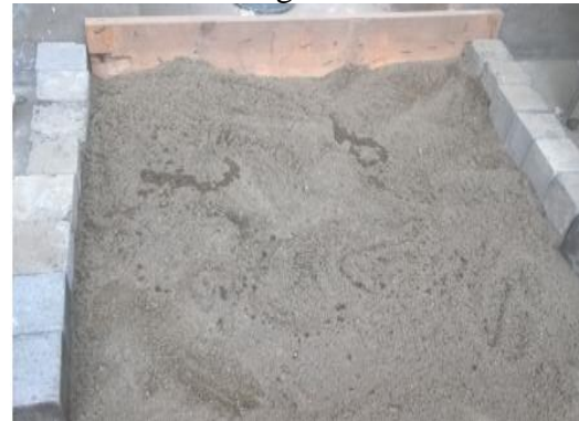
Figure 3.2 : Coal bottom ash
