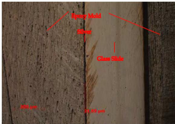
Figure 1.1 Optical cross section of the V2 silver on a glass slide in an epoxy mold.
