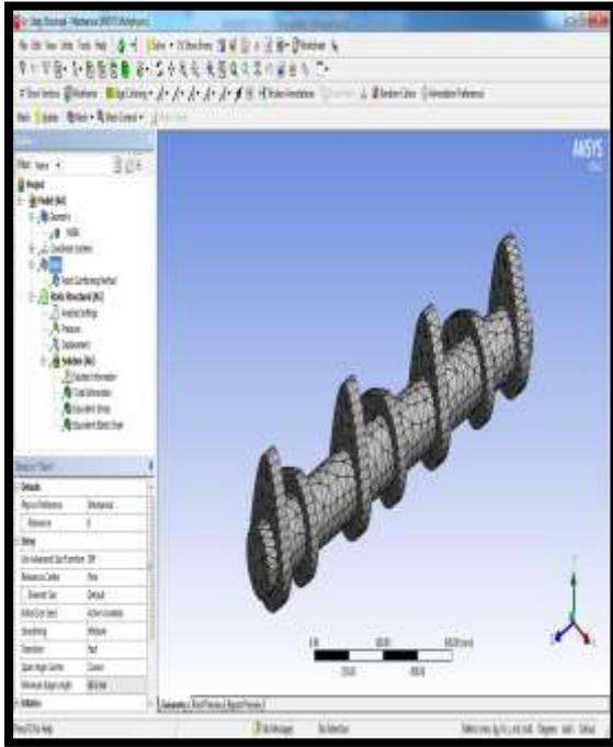
Select static structural right click on → insert → pick rotational velocity and stuck assist → Select displacement → select required area → click on practice → positioned X,Y,Z factor 0 →
